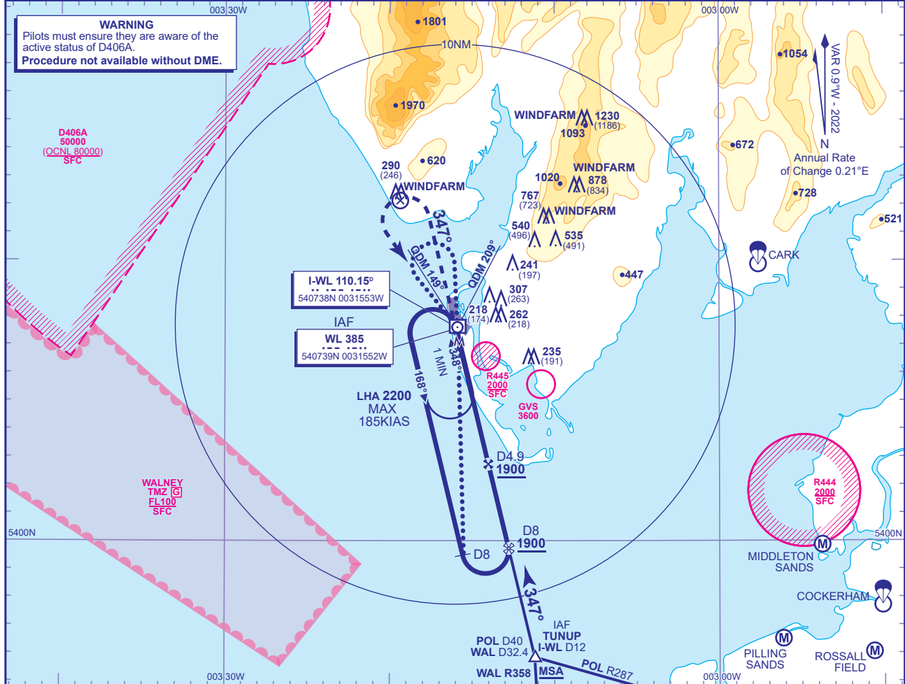
RECOMMENDED PROFILE Gradient 6.12%, 372FT/NM
